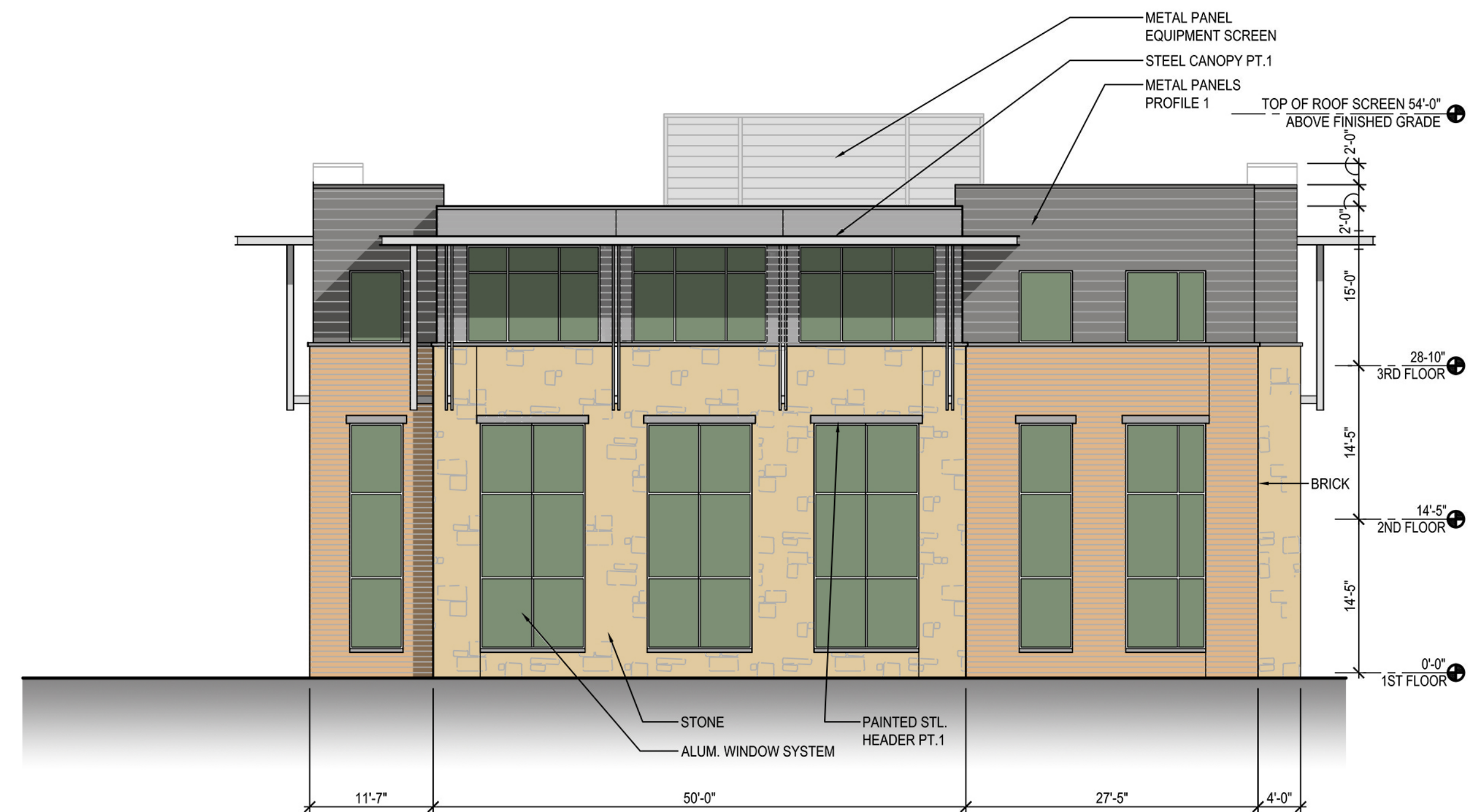
1 Building 1 - North Elevation Scale: 3/32"=1'-0"
